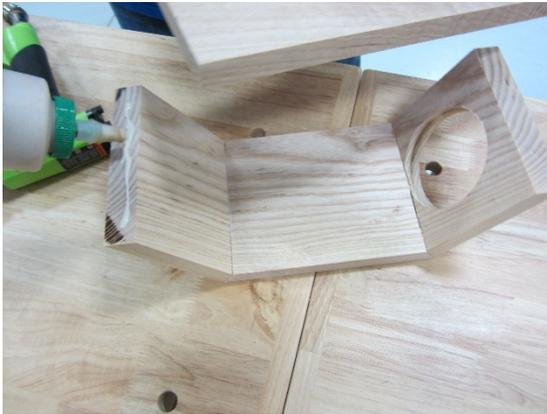
11. Glue and pin nail the top 14" piece to the ends.
