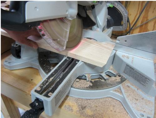
8. Cut a piece 7 ½" long from long point to long point with that 30 degree angle on both sides. This will be your bottom piece.
