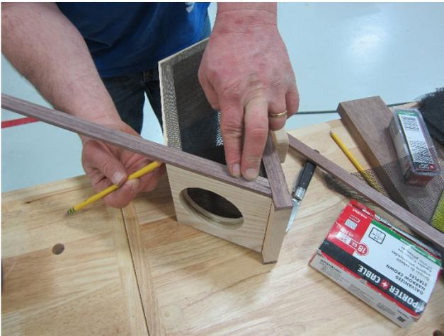
14. Pin nail the strips to the critter ark over the screen to cover up the staples.
