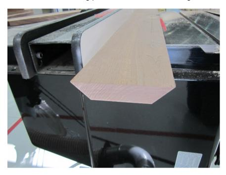
Next, using a miter saw, cut 4 pieces a 4 <sup>3</sup>/<sub>4</sub>" in length.
