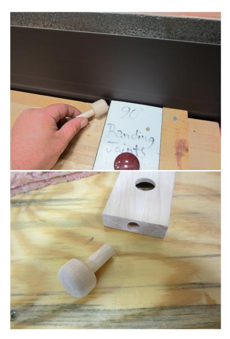
Now you want to cut the  $\frac{1}{2}$ " dowel so there is 1  $\frac{1}{2}$ " sticking out of the bigger dowel and glue and hammer it into the front of the slide. Your slide is finished.
