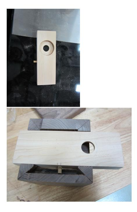
Next drill a  $\frac{1}{2}$ " hole in the center of the front end for your handle. Go in  $\frac{3}{4}$ ". Using a 1 1/8" dowel rod (or similar), drill a  $\frac{1}{2}$ " hole in the center of it going in only 5/8". Round the outer edges of it on the side with the hole, then glue and hammer in a  $\frac{1}{2}$ " dowel into the bigger dowel.
