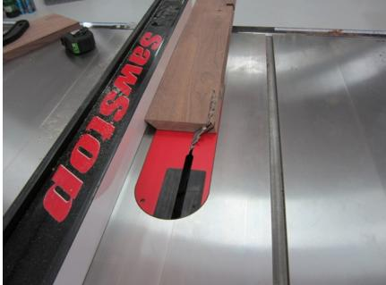
Then run the other side of the board back through so you have a 45 degree angle on both sides with the long points of the 45's measuring 4  $\frac{1}{2}$ " between them.
