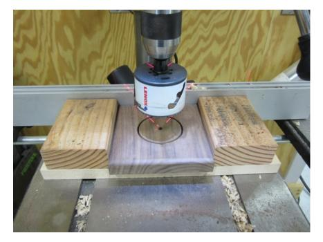
Optional: You can drill a 1  $\frac{1}{2}$ " hole in the center of the other piece which becomes the base, then get a 1  $\frac{1}{2}$ " rubber plug and use the lower half of the dispenser as a piggy bank.
