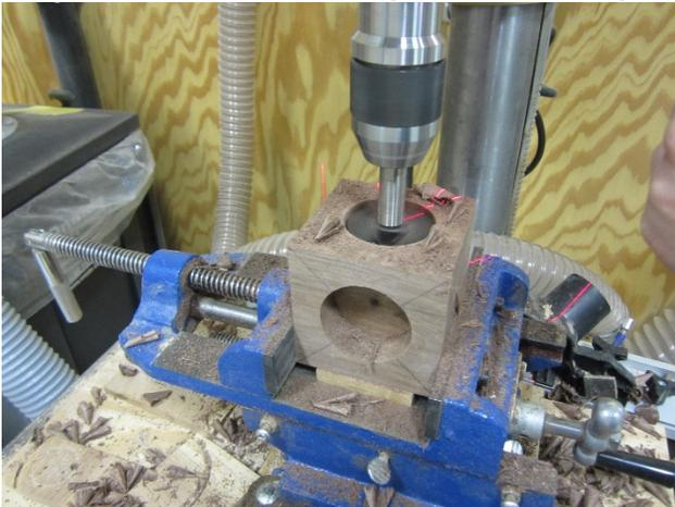
7. Now lower the drill bit slowly until there is just a little piece of wood holding the corners of the inside cube.
