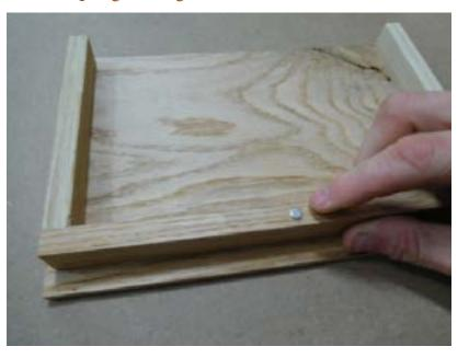
8. Clamp sides together with the beveled piece facing down in between sides. Attach your leather bindings with tacky glue 1" from ends.
