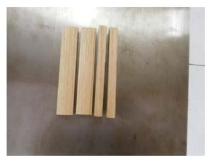
4. Cut one 10 ½"x 2"x ¼" piece of wood. Set tablesaw at a 5-degree to bevel the 10 1/2" edges.
