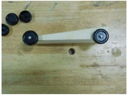
Place axle through tire into the wood by hand. \*Note\* axle should be able to be
