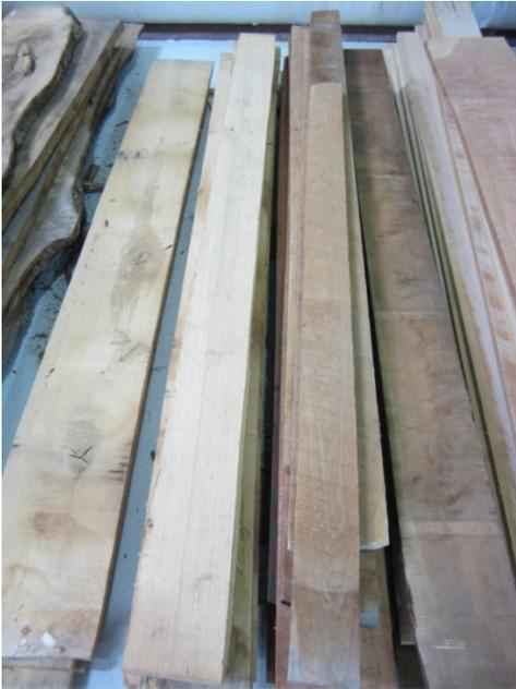
2. Plane the boards to a thickness of  $\frac{7}{8}$ " and cut poles to  $1\frac{3}{4}$ " wide by 7ft long.
