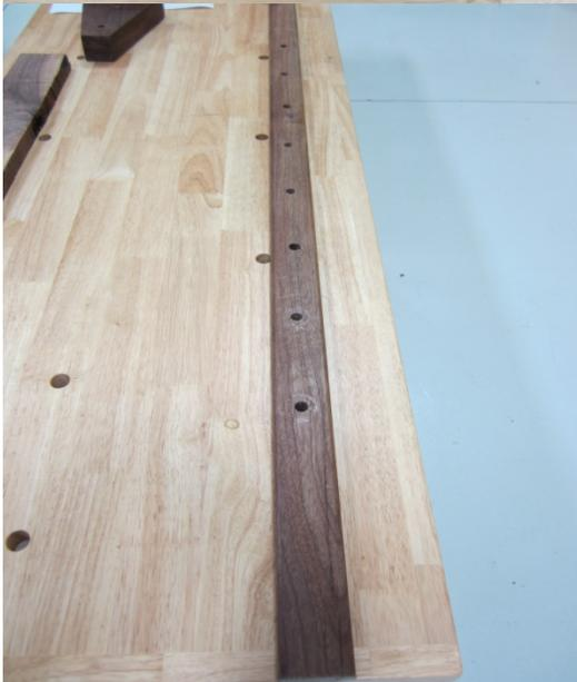
4. Cut out 4 boards for the foot rests that are  $\frac{7}{8}$ " thick by 7" tall and width being 5" at top tapered to  $1\frac{3}{4}$ " at the bottom. Also cut out two tops  $\frac{7}{8}$ " thick by 5" long and  $3\frac{1}{2}$ " wide.
