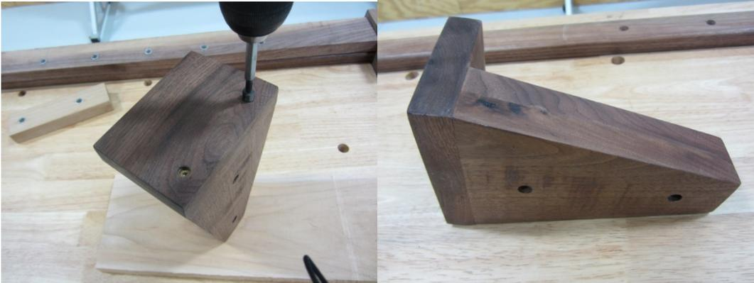
6. Drill two holes on each of the foot rests. Find the center on the side of the foot rest and measure 2" down and 2" up from center for your holes. These holes should have the same spacing and have the same alignment as on your pole.
