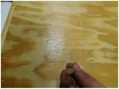
6. Slide the dowel into the hole, flat side facing toward wedge, and adjust depth until you get your desired sound. Super glue the dowel in place and cut off excess.
