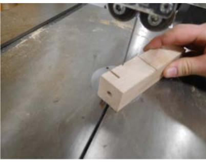
4. Cut from appropriately 1 7/8" over, down to bottom of first cut, so that you remove a v shaped notch out of the block. (Wedge should be 30 degree).
