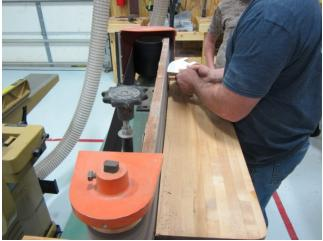
8. Using a ¼" drill bit, drill holes for dowels. When drilling be sure to drill holes straight and not at an angle. Drill down just enough to hold the dowel secure, about 1/4" to 3/8".
