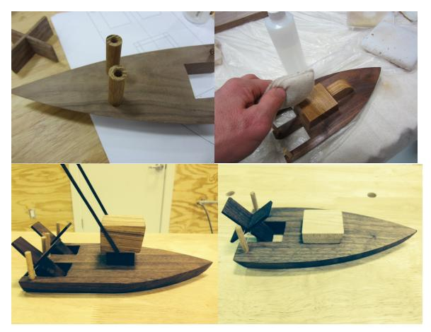
11. Insert ¼" dowels for propeller mount. Be sure to wipe off excess wood glue with wet rag.
