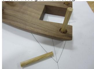
12. Cut propellers out. 1/8" thick by 3" long by 1 3/16" wide if using a one propeller boat, and only 1" wide if using a two propeller boat. Cut a 1/8" slot in the middle of each fin going halfway across. Slide two fins together using these slots and glue together. Taper ends of propeller slightly (this makes it less likely to bind). Option- If you drill
