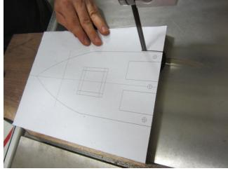
6. Reset jig saw or band saw table to square. Cut the back of boat and the propeller bay.
