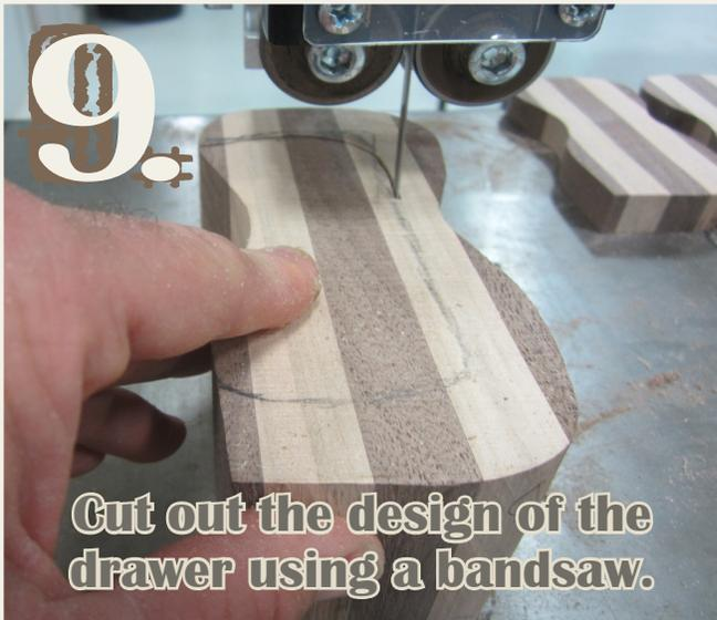
Cut out the design of the drawer using a bandsaw.
