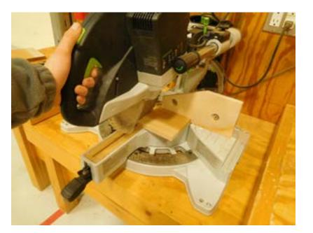
8. Cut ½"off the corners of the bottom piece to allow for ventilation.
