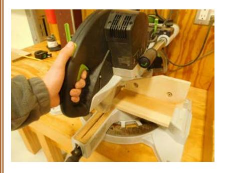
7. Cut the bottom 5 ½" minus the thickness of the board.
