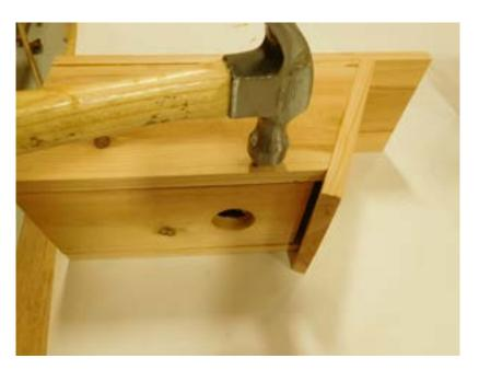
12. We used a nail and a neodymium magnet centered at bottom to hold the front shut. \*\* Note \*\* Drill bit size depends on the magnet size and nail size you have chosen.
