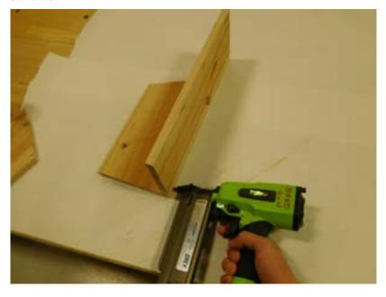
11. Attach the front with two nails in line with each other, 7" from the bottom. This should allow your front to swing open.
