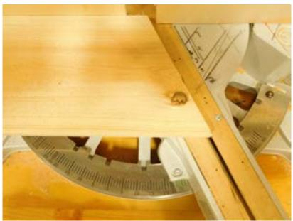
4. Cut a piece  $7 \frac{1}{4}$ " x 5  $\frac{1}{2}$ " from long point to long, point with a 25-degree bevel on one end for the roof.
