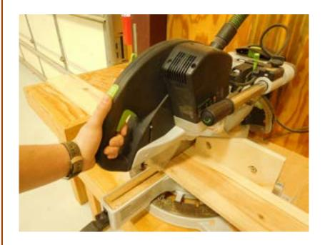
3. Cut two pieces 12" x  $5 \frac{1}{2}$ " from long point to long point with a 25-degree angle for the sides.
