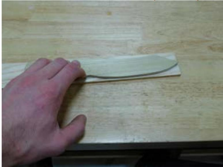
3. Using The band saw cut out the blade portion of the knife only.
