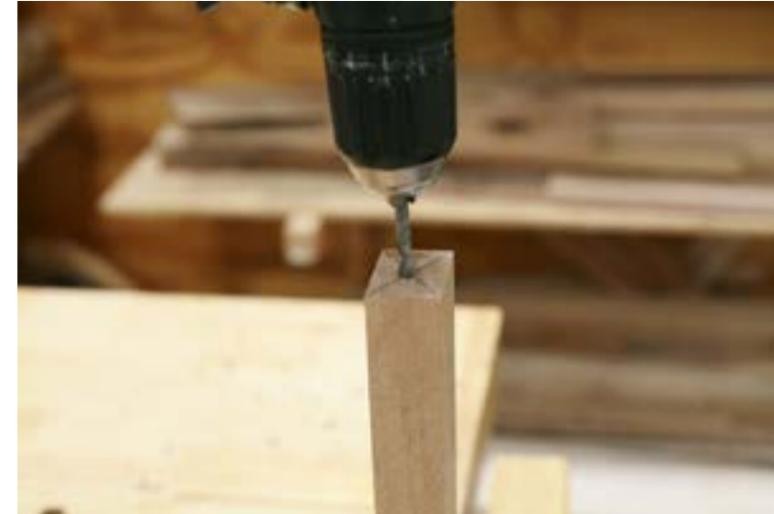
27. Find the point of balance point on the bottom of your whirligig and drill a 3/16" x 1" hole.
