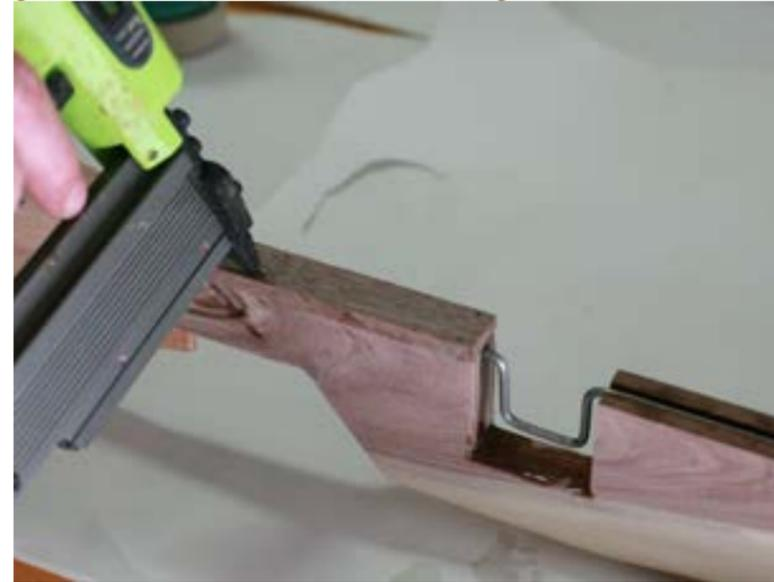
18. Slide the fan over the wire, then bend the wire over and staple in place on the front of the hub, leaving a 1/8" gap between the main part of the whirligig and the hub.
